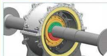
步骤六 Step 6 胀套紧固并与转子连接 Fix the expansion sleeve and connect with the rotor
